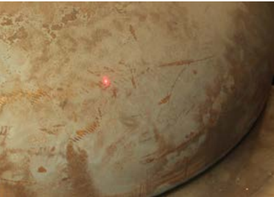
Laser triangulation measurement of the surface enables adaptation of the theoretical 3D cutting path to the deviations of the raw material.
