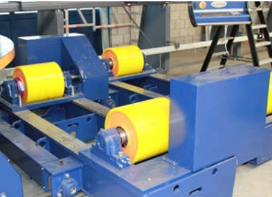
The supports can be motorised to easily move a shell along the rails.
